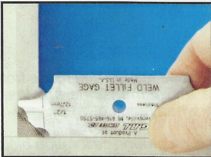
CHECKING FILLET THROAT SIZE
